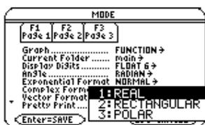
You can enter a complex number at any time, regardless of the Complex Format mode setting. However, the mode setting determines how results are displayed.
