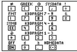
The keyboard map displays shortcuts that are not marked on the keyboard. As shown below, press ◆ and then the applicable key.
