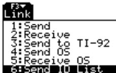
The sending unit adds a copy of its unique ID number to the collection unit's ID list. The sending unit always retains its own ID number, which cannot be deleted from the device.
