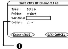
**Note:** If you type the name of an existing variable, its contents will be replaced.
