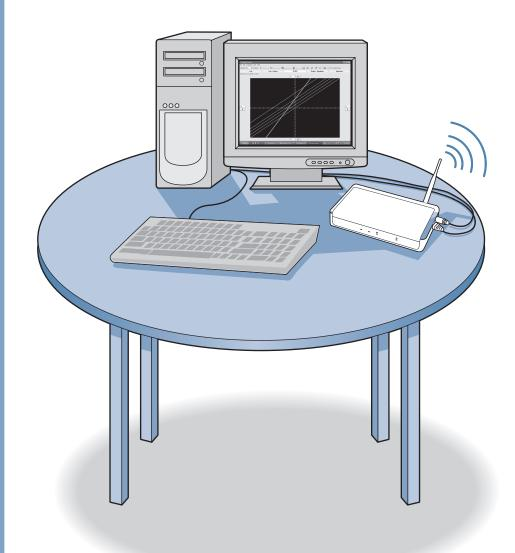
**Network Hubs** communicate with access point. TI calculators connect to hubs.
