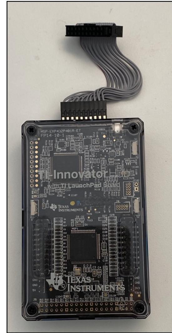
Step 4: Lift up the cable and push the TI-Innovator Hub out of the Rover.
