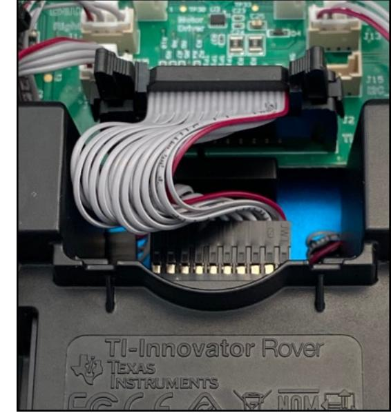
Step 2: Push the connector onto the pins. The clips on the side will lock the connection.
