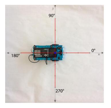
Rover programs set the initial position as the origin and the heading as 0 degrees measured from the x-axis.
