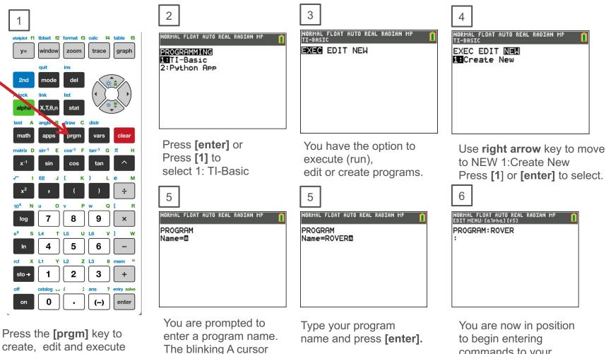
The blinking A cursor shows that you are in alpha entry mode. The green alpha labels on the keys are active.
