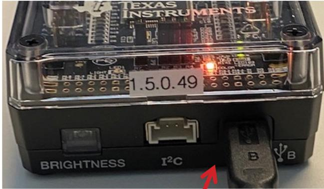
**Note:** The Hub is powered by the calculator. When the cables are connected the Hub goes through a brief “boot-up” process. During the boot-up the RGB LED displays a color that indicates the Hub firmware release, in this case, orange.
