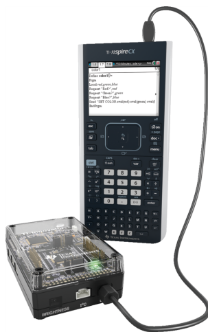
Hub collegato a palmare TI-Nspire™ CX
