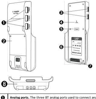
**Analog ports.** The three BT analog ports used to connect analog sensors. The other side of the cradle has two digital ports for digital sensors.
