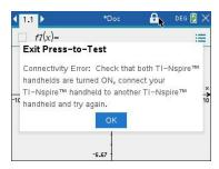
The handheld does not exit Press-to-Test mode until it restarts. If you disconnect the cable before the restart begins, the handheld remains in Pressto-Test mode.
