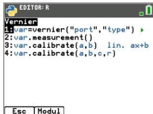
The "vernier()" function has two helper prompts – for the port and for the type of sensor attached.
