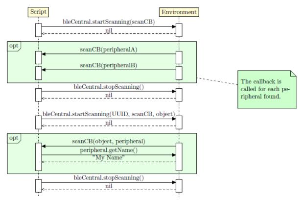
Figure 20.1: Bluetooth® LE Scanning Procedure
