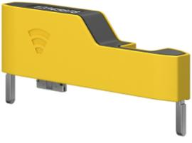
A yellow, L-shaped wireless network adapter with a black top surface and two silver legs. The TI logo is visible on the yellow surface.                                          | Attaches to the TI-Nspire™ CX and TI-Nspire™ CX CAS handhelds to enable wireless communication over a 2.4GHz band.         |
