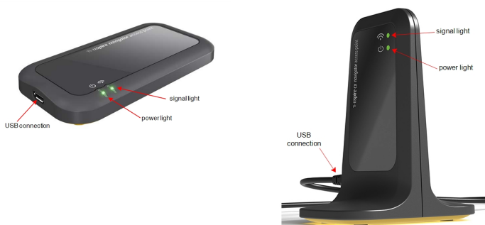
TI-Nspire™ Navigator™ access point TI-Nspire™ CX Navigator™ access point
