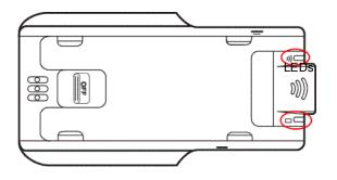
The  $\widehat{\mathbf{T}}$  LED indicates network activity. The  $\mathbf{D}$  LED indicates battery-charging status.
