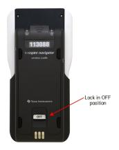
2. To attach the handheld, face the screen upward and slide the handheld onto the top of the wireless cradle. Be sure that both sides of the handheld are inserted into both of the side guides.
