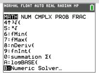
**Example 1:** To solve the equation 3x+5=5x-9, press math and select B:Numeric Solver, and press enter. Type the left side of the equation, 3x+5, into E1: and the right side of the equation 5x-9 into E2. Move between E1 and E2 by using the arrow keys, and press the graph key to select OK. You can type in a value for x or have the calculator solve this for you. Next, press the graph key again to solve. Notice once the equation is solved, there is a dark square to the left of the variable.
