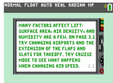
7. On page 2.2 there are three different modes for you to explore. Use the right/left arrows to change between modes. Note: you can only change modes when the flaps and slats are not extended. Press the up/down arrows to extend/retract the flaps and slats. The flaps and slats are parallelograms with the height equal to the extension. The width of the slat is 12.5 meters and the width of each of the flaps is 5 meters.
