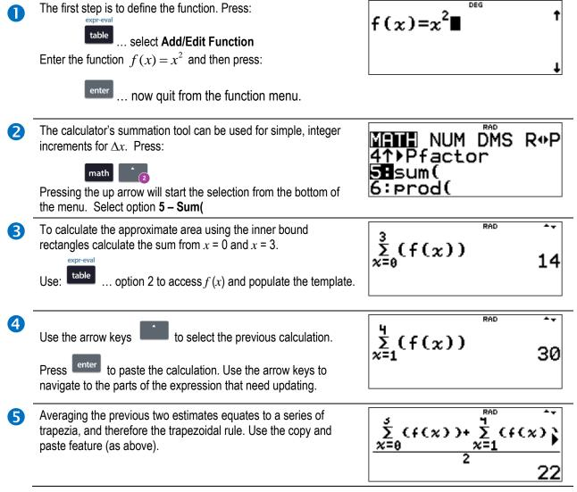
The summation tool use integer increments. It is possible to manipulate the expression to work for non-integer values. In this example start at x = 0 and go to x = 39, calculate f(x/10) then multiply by the column width 0.1. Similarly, start at x = 1 through to x = 40, however the calculator lists is a better option here. (Refer Part 2)
