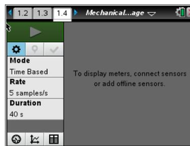
4. Next, zero the force sensor (**Menu > Experiment > Set Up Sensors > Zero**). Then, use the string to connect the cart to the hook on the bottom of the force sensor. (Make sure the switch on the force sensor is set to the correct range. The range you use will depend on the mass you use.) Let the cart hang from the force sensor without touching anything. Once the weight reading on the force sensor has stabilized, record the weight of the cart on paper.
