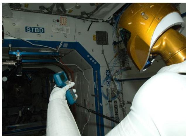
Figure 2: R2 holds an instrument to measure air velocity during a system check-out on the ISS
