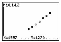
To use the regression capabilities, press STAT > to access the CALC menu. Select 4:LinReg(ax+b), since the graph appears to best be described as linear.
