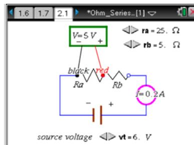
Then measure voltages across resistors by connecting wires properly.
