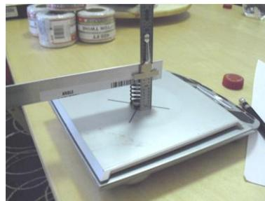
7. Pour more water into the bottle until the spring is a little over half compressed. Measure and record the new length and the weight from the scale.
