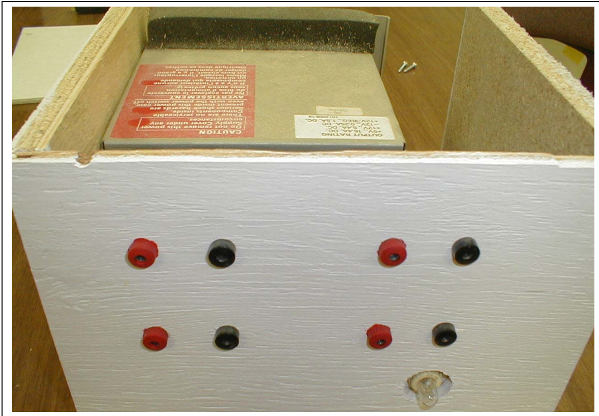
Figure 1A: Computer Power Supply (Front Panel)
