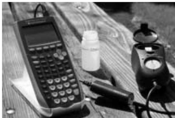
tissue and place it in the Colorimeter. After closing the lid, wait for the value displayed on the calculator screen to stabilize and select (Keep).
