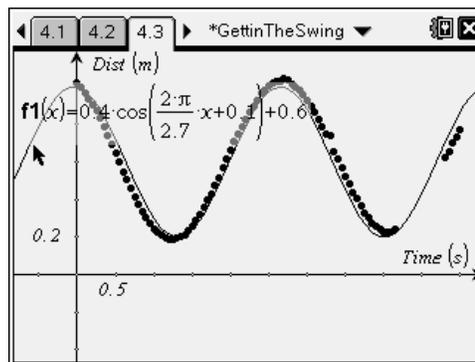
Be sure to use a smooth ball so that the sonic pulse is reflected off the surface well.
