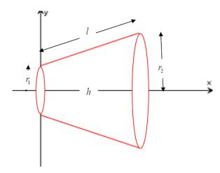
b. Show that the surface area of a truncated cone (or frustrum) with inner and outer radii of  $r_1$  and  $r_2$  and slope length l is given by  $S = \pi \left( r_1 + r_2 \right) l$ .
