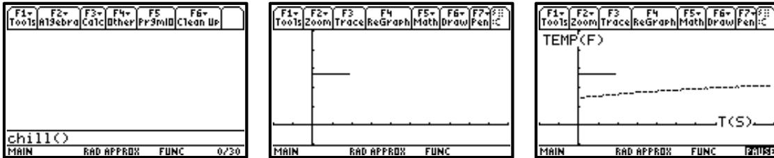
First use the CBL to determine the room temperature,  $T_s$ . Then collect temperature data following the directions within the program. Place the thermometer in ice (or hot) water for a few seconds. Then remove the thermometer and take data readings as it warms (or cools) to room temperature. Finally, from the menu, select QUIT, then [ENTER] to return to the home screen.
