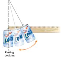
motion sensor, position it 1 meter from the can along the path of the swing; the program will collect the maximum distance from the resting position for 30 swings.
