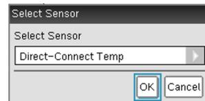
Sensors that do not auto-ID must be set up everytime they are used and will not be identified by the software when opening a saved file.
