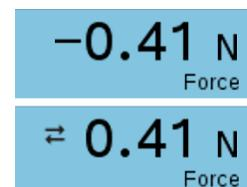
Press **[menu]** then choose Set Up Sensors ► Reverse from the
