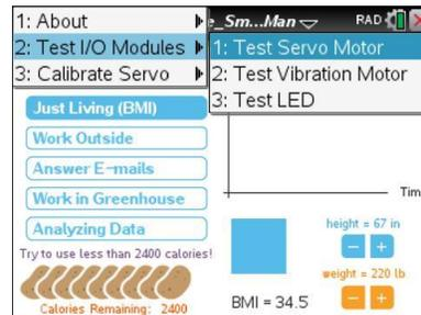
**Teacher Tip:** Over time, the Servo Motor may not operate correctly and will need to be recalibrated. Go to **menu> Calibrate Servo> Calibrate Servo**. If the Servo does not move, then it’s already calibrated, If the servo is moving, use a screwdriver to move the potentiometer in the back of the motor until it stops. If you need more assistance, contact Customer Support [education.ti.com/support](http://education.ti.com/support).
