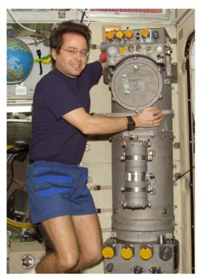
Figure 3: Astronaut Daniel W. Bursch working on the Elektron Oxygen Generator in the Zvezda Service Module on the ISS
