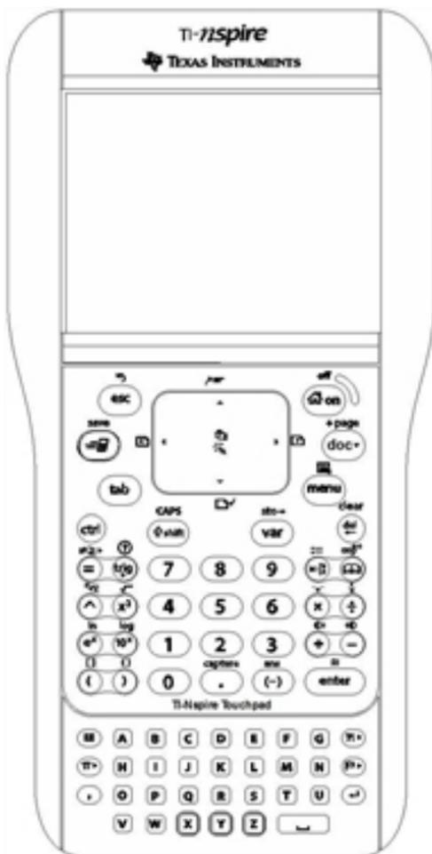
**(on)** Turns on the handheld. If the handheld is on, this key displays the home screen.
