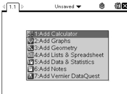
3. Press **(menu)** to display the Application menu, which lists the options for working with the current application.
