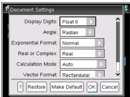
2. Press **(tab)** to move through the list of settings. Press **(up arrow)** to move backward through the list.
