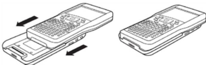
3. Press firmly to make a good connection. When properly connected, the *TI-Nspire™ handheld appears to be sitting on top of the cradle.*
