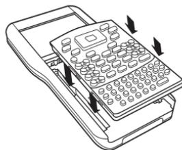
5. When the keypad is properly seated on the handheld, push the keypad toward the display screen.
