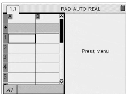
3. Press **(ctrl)** **(tab)** to move between panes. Bold lines around the pane indicate that the pane is active.
