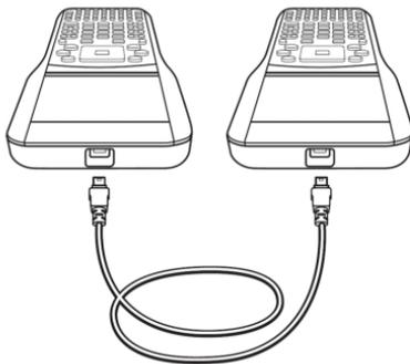
The USB port is located on the top of the TI-Nspire™ CX handheld on the right side when holding the handheld with the screen facing you.
