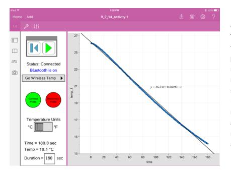
Possible results from project evaluation. The Go Wireless Temp sensor was placed in the bottle shown above and put in a refrigerator for 3 minutes. Although this data is not perfectly linear (nor should it be), a linear regression may be a good method of analysis and an appropriate level of mathematical modeling for students.
