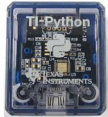
Front view - Port for connecting one end of the provided cable to the TI-Python Adapter port labeled B.
