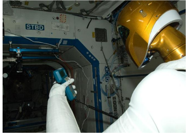
Figure 2: R2 holds an instrument to measure air velocity during a system check-out on the ISS
