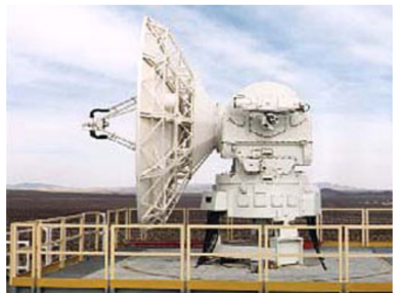
Figure 2: WATR instrumentation radar
