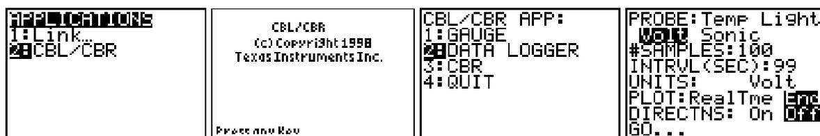
7. Once set up, with the item plugged in with the penny and washer and the CBL™ turned on with the voltage probe in **CH1**, highlight the word **GO** and press **[ENTER]** to start the data collection. Set the experiment aside and come back at the end of the set time. You can determine this by multiplying the number in **#SAMPLES** by the number in **INTRVL(SEC)**.
