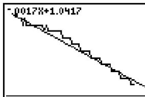
16. To look at the rule (equation) created from the **Manual-Fit** calculation, press **[Y=]**. **Y1** is the voltage of the battery created by the item studied (Lime). **X** is the time in minutes when this voltage occurs. The value of 1.0417 in the sample screen below is the voltage at time zero (this should be close to the voltage that you got from the first data collection). The number in front of **X** is the rate of decay of voltage in minutes (in this case  $-0.0017$  volts per minute).
