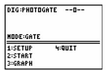
You are now ready to launch your paper ball projectile. Have one student hold the Photogate sensor up. Launch the paper ball projectile so that it passes directly through the Photogate sensor when released (make sure the spoon does not pass through the sensor).
