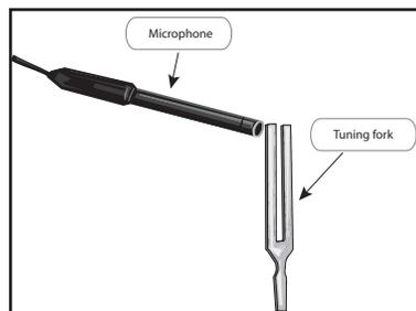
(Note: *Never* strike the tuning fork on a hard surface; it may change the waveform of the tuning fork.)
