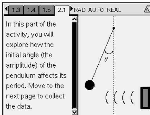
**Step 3:** Students should repeat the data collection for initial angles of 10° and 15°. They should keep the mass of the pendulum bob and the length of the string the same for all three trials. They should record the period of the pendulum in each case in the *Lists & Spreadsheet* application on page 2.3.
