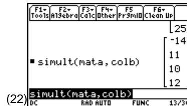
Referring to the matrix equation for the circuit as shown below, the values returned by `simult()` correspond to the variables in the first column vector. The solution is  $v1=-14$  V,  $v2=11$  V,  $v3=10$  V, and  $i25=12$  A, the same answer as in Topic 2.
