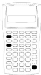
To store a constant for use in repetitive calculations, enter a number and an operation, and then press  $\boxed{2\text{nd}} \boxed{[K]}$ .
