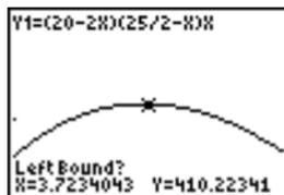
2. Press  $\boxed{\blacktriangleleft}$  to trace along the curve to a point to the left of the maximum, and then press  $\boxed{[ENTER]}$ .
