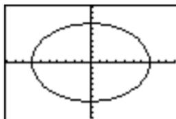
**Tip:** When you use **Circle(** on the home screen or from a program, the current window values may distort the drawn circle. Use **ZSquare** (Chapter 3) before drawing the circle to adjust the window variables and make the circle circular.
