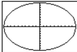
3. To adjust the display so that each pixel represents an equal width and height, press  $\boxed{ZOOM} \boxed{5}$  to select **5:ZSquare**. The functions are replotted and now appear as a circle on the display.
