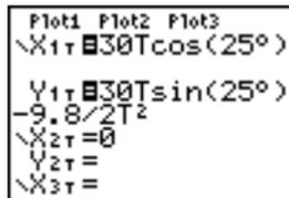
5. Press **VARS**  $\rightarrow$  to display the VARS Y-VARS menu. Press **2** to display the PARAMETRIC secondary menu. Press **2** **ENTER** to define **Y2T**.
