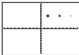
**Note:** If you specified *mark* to turn on a point with **Pt-On(**, you must specify *mark* when you turn off the point with **Pt-Off(**. **Pt-Change(** does not have the *mark* option.
