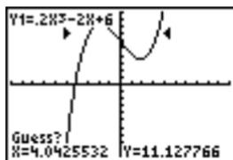
4. Press  $\leftarrow$  or  $\rightarrow$  (or enter a value) to select a point near the zero of the function, between the bounds, and then press  $\text{ENTER}$ .
