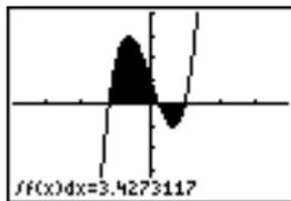
**Note:** The shaded area is a drawing. Use **ClrDraw** (Chapter 8) or any action that invokes Smart Graph to clear the shaded area.
