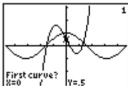
2. Press  $\downarrow$  or  $\uparrow$ , if necessary, to move the cursor to the first function, and then press  $\text{ENTER}$ . **Second curve?** is displayed in the bottom-left corner.
