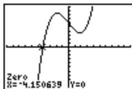
The cursor is on the solution and the coordinates are displayed, even if **CoordOff** format is selected. To move to the same x-value for other selected functions, press  $\uparrow$  or  $\downarrow$ . To restore the free-moving cursor, press  $\leftarrow$  or  $\rightarrow$ .
