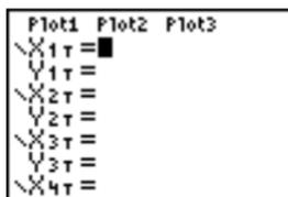
In this editor, you can display and enter both the **X** and **Y** components of up to six equations, **X1T** and **Y1T** through **X6T** and **Y6T**. Each is defined in terms of the independent variable **T**. A common application of parametric graphs is graphing equations over time.
