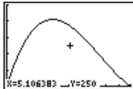
3. Press **[◀]**, **[▶]**, **[▲]**, and **[▼]** to move the free-moving cursor to the apparent maximum of the function.
