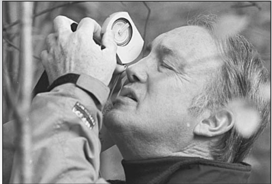
Out on a limb: Bob Leverett uses a clinometer to gauge the height of a tree near Syracuse, N.Y.
