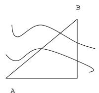
A surveyor at point A measures the angle shown in the triangle at point A. The surveyors also know the distance from point A to the point directly across the river from point B. So with that information can they find the distance across the river?
