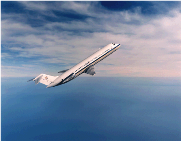
Figure 1: C-9 jet going into a parabolic maneuver.
