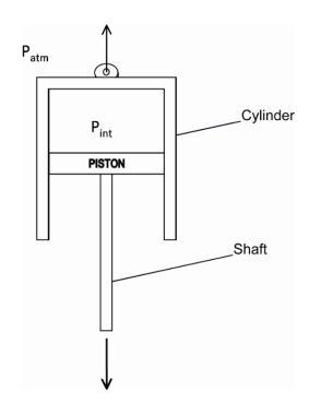
Figure 2: A model of ARED showing the piston/cylinder assemblies
