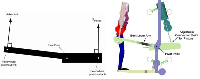
Figure 4: A side-view illustration of ARED showing the bent lever arm
