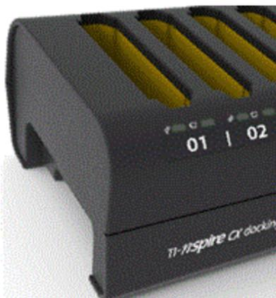
To determine the status of the handheld's batteries, look at the Battery Status LED indicator for the slot under the handheld. The Battery Status LED Indicator is located to the right of the battery symbol (
