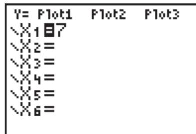
Place the cursor so that it is positioned on the equal symbol. Select the greater than or equal to symbol, ( $\geq$ ), by pressing  $\boxed{ALPHA} \boxed{F5}$ .
