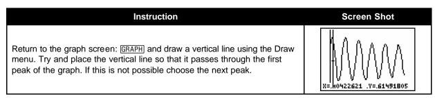
Press 2nd MODE to return to the home screen. You can recall the value for X by pressing  $X,T,\Theta,n$ . The X axis represents time. The phase shift in the data above is approximately 0.4 seconds. Determine which parameter in the equation:  $Y_1=A\cos(B(X-C))+D$  is responsible for the phase shift.
