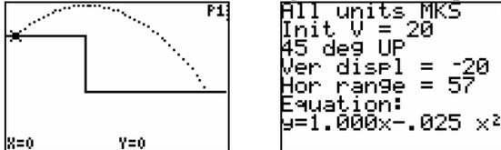
When viewing the graph screen above, the left and right arrow keys can be used to move along the projectile's path. The (X,Y) coordinates of the projectile are displayed as you move along the path. The origin is at coordinates (0,0). The graph screen is rescaled for every problem to make the best use of the screen. No two subsequent simulations are likely to be at the scale.
